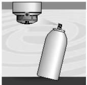
After installation, the Smoke Switch must be tested for correct operation using the test aerosol. When carrying out tests, be sure to follow the safety instructions printed on the can of Test Aerosol 918/5.
